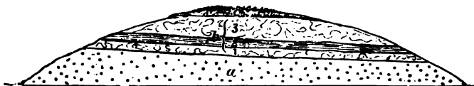
a. Lower Sands. b. Ironstone. c. Soil with flints from the drift.
